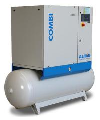
Description The ALMiG COMBI series is a belt driven compressor inside an enclosure with electrical cabinet and pressure switch control. The system is designed for belt drive between the motor and compressor for almost zero-loss power transfer and the greatest possible efficiency.
